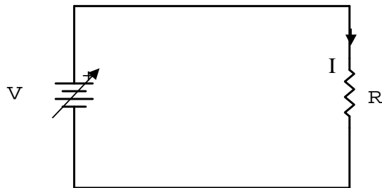
Fig. 1.1: Circuit for verification of Ohm's Law
